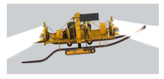
These two machines work together to unload and deposit the rails alongside the embankments in order to prepare the site for the next machine.
