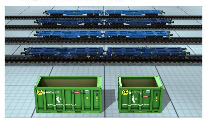
The arrangement of the containers for transport by freight wagons is flexible, although predefined locations are provided. These containers are, as in reality, fixed to anchoring points present on the transport wagons.
